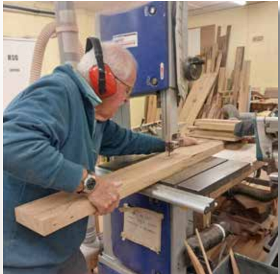
Graham Smith cutting the component boards using one of the men's shed's band saws.
