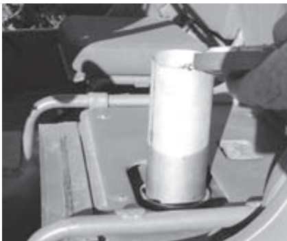
Fuel filler, under passenger seat
